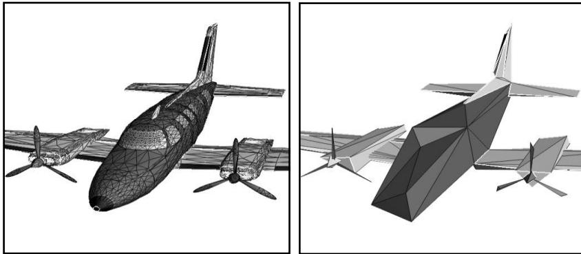
Figure 1: Flexible strategy for reducing the complexity of models. Methods for reducing the number of vertices used to describe a geometric model can be used to generate a spectrum of models from an ideal model to progressively simpler models. The fully detailed model (left) is described by 6,795 vertices. The simplified model (right) is described by 97 vertices.
