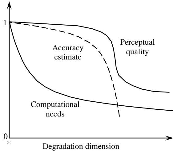
Figure 5: In pursuit of perceptual costs and computational savings. We seek to move beyond information about the relationships between estimates of accuracy and measures of simplification, to gain a better understanding of the overall perceptual losses and computational savings as graphical content is degraded along one or more dimensions.
