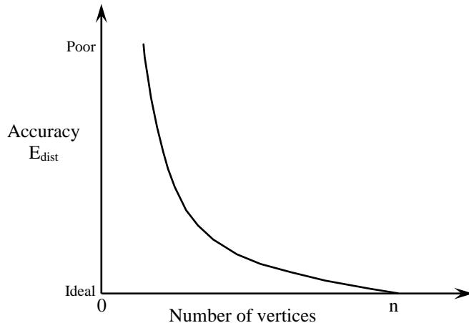
Figure 2: Tradeoff between size and accuracy. The graph displays how the relationship between a measure of model accuracy based on an energy quantity ( $E_{dist}$ ), defined as the total squared distance of the points in a reduced model from the fully detailed mesh describing the ideal model, varies with the size of the model produced by the progressive mesh approximation procedure.
