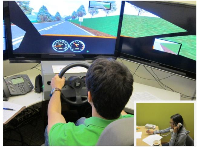
**Figure 1:** Participant driving the STISIM simulator. The simulator provides a console with speedometer, steering wheel with turn signals, and traditional brake and accelerator. Three 47" screens generate an impression of driving a vehicle. The driver used a speaker phone system (center left) to converse with the remote caller (inset).
