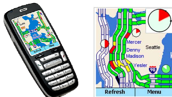
Figure 5: Smartphone application. Clock graphics are used to display time until a congested bottleneck will clear (red) and the time until a bottleneck that is currently open will become congested (green). Inset: close up of prediction, showing confidence as represented by the standard deviation.
