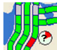
Figure 7: Use of a question mark annotation to relay to the user that prediction may be unreliable in the situation at hand, based on inference with a context-sensitive reliability model for a bottleneck.
